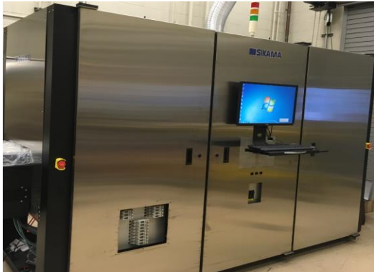
Figure 1: EA-enabled prototype furnace for production-scale wafer bump reflow
