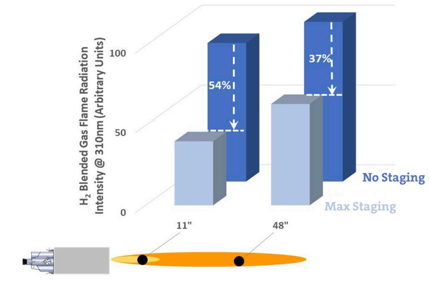
**Figure 5** shows additional emission spectral measurements of the hydroxy (OH) radical measured at 310 nm. The OH radical provides an indication of progression and reactivity of the combustion reaction. The measurements were taken using 30% H<sub>2</sub>/70% NG fuel blend at two locations, 11" (0.3m) and 48" (1.2m) from the hot face of the burner block (as shown on the x-axis of the graph). The measurements were taken at two burner conditions, both with
