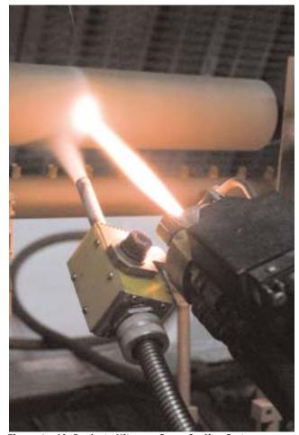
Figure 4: Air Products Nitrogen Spray Cooling System Air Products' cryogenic spray nozzle installs easily on any thermal spray gun to help cool parts twice as fast as air cooling alone, which allows thermal spray operators to work faster and more efficiently with less wasted powder, process gas, and booth time.
