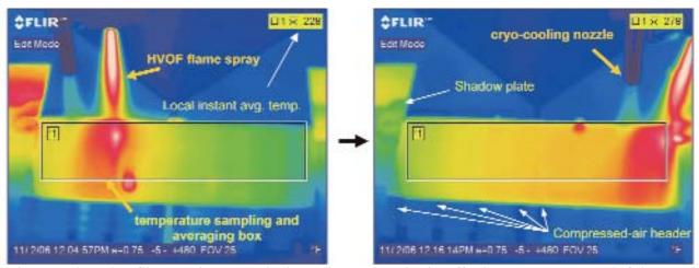
Figure 3: Thermal profiles at various stages in the coating process, showing effective temperature control of the coated surface with cryogenic cooling (a) Start of spraying pass (b) End of spraying pass
