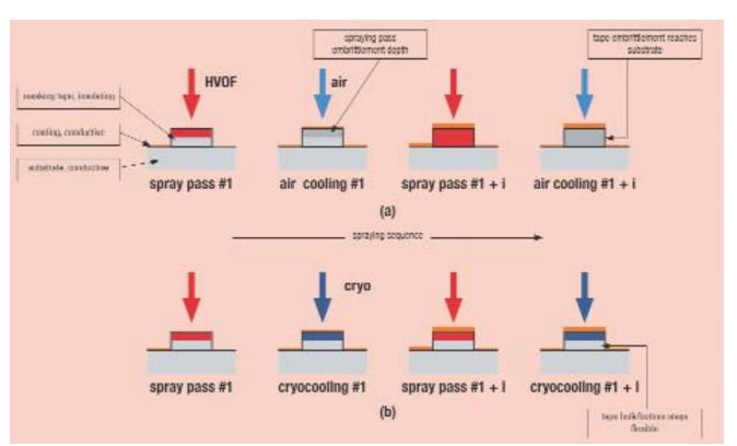
Figure 2: Effects of cooling on silicone-based masking tapes during HVOF spray (a) Air cooling (b) Cryogenic nitrogen vapor cooling
