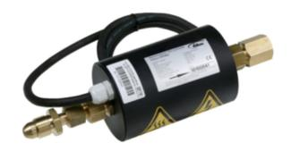
The CO<sub>2</sub> Heater is designed to vaporise liquid carbon dioxide from syphon type CO<sub>2</sub> cylinders where a greater flow rate is required than is available from standard gas off-take cylinders.
