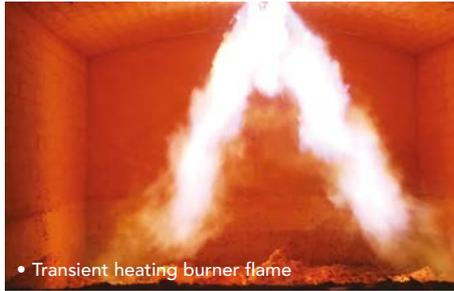
• Transient heating burner flame
