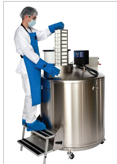
**Use the correct equipment.** Because of the large amount of gas created by evaporation of liquid nitrogen, for storage and transport do not use anything except equipment specifically designed for the purpose. Unvented containers must not be used. Many materials become extremely brittle and likely to fracture at liquid nitrogen temperatures.
